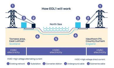
Converter stations and substations are required onshore at each end. Metlen Energy & Metals and GE Vernova are responsible for the design and build of the convertor stations.
